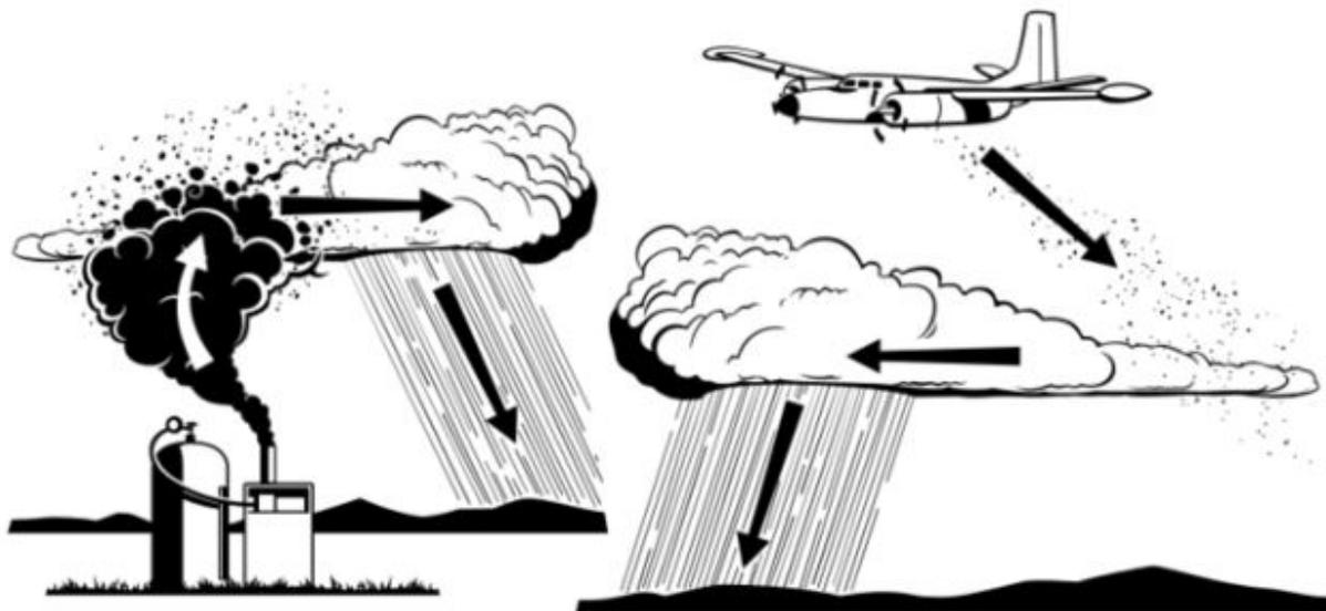
**Figure 5:** Cloud seeding from a plane or ground-based generator. (Source: Wikimedia Commons)
