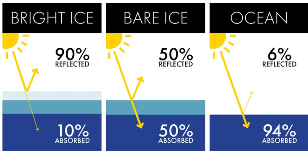
**Figure 3:** Ice911's material mimics bright ice to reflect heat -- ideally keeping more ice in the Arctic. (Source: Ice911)
