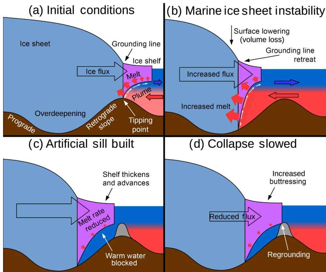
**Figure 8:** Schematic diagram of marine ice sheet instability and mitigation with an artificial sill. Brown represents bedrock, light blue represents the grounded ice sheet, purple represents the floating ice shelf, and gray represents an artificial sill. Ocean temperatures are drawn to represent the typical stratification faced by marine-terminating ice streams: warm salty water at depth (red) and cold fresh water (blue) near the surface. (Source: Wolovick et al, 2019)
